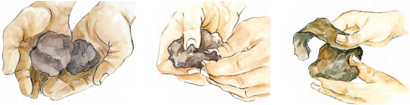
Figure 3-9: Texture by “feel” test
