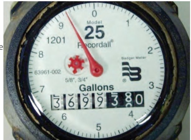
Figure 1-11: Straight-reading meters in gallons (upper) and cubic feet (lower)
